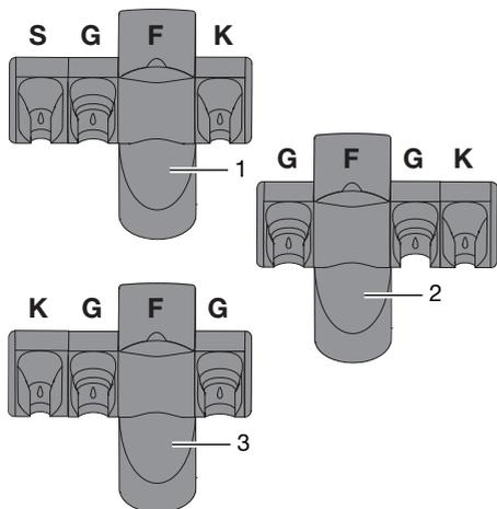
Fig. 4: 4-fold hose manifold Comfort
