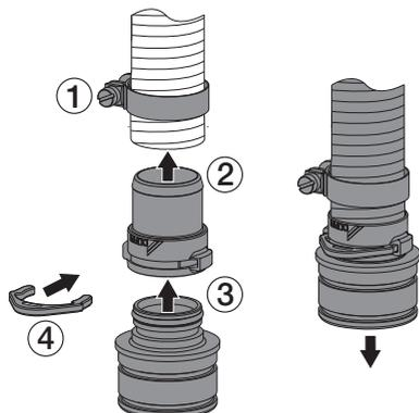
*Connect the rinse hose and lay correctly:*
