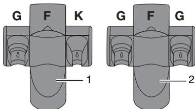
Fig. 3: Triple hose manifold Comfort
