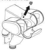
Insert the screwdriver horizontally through the opening and tighten the screw.
