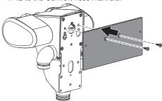
Mount the adapter plate with the Comfort hose manifold using a countersunk screw M4 x 12 and M4 hex nut to the mounting plate.
