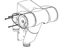
Pressed the section marked from both sides in order to take the element apart.
