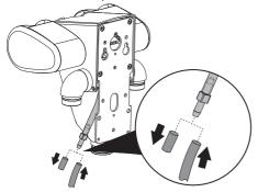
Lay the rinsing unit hose, ensuring as far as possible that it is parallel to the central suction hose. Attach the hose with the clip to the central suction hose.
