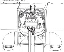
> Disconnect the cable in the filter element.
